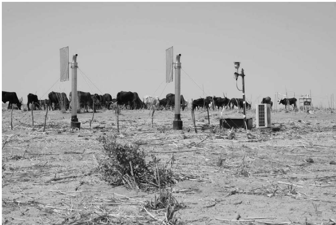
Figure 4. The two IPC samplers standing above the buried container (note the access trap to the container on the right of the samplers and the air conditioning system) and the PM10 Rupprecht and Patashnick Inlet. The field sparsely covered with millet straws is typically grazed by cows during this period of the year.
