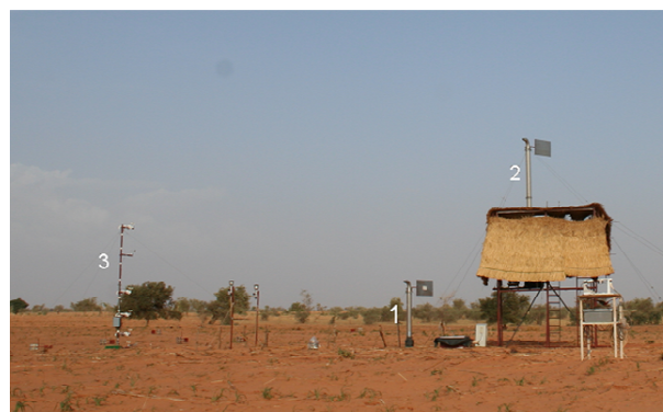
Fig. 1. View of the experimental site showing the two sampling systems located at elevations of 2.1 m above the buried container (1) and of 6.5 m on the tower (2), and the meteorological mast (3).
